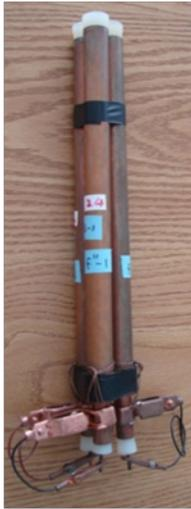
Figure 3 - 4 Experiment Apparatus (surface area over volume = 0.047 cm<sup>2</sup>/ml)
