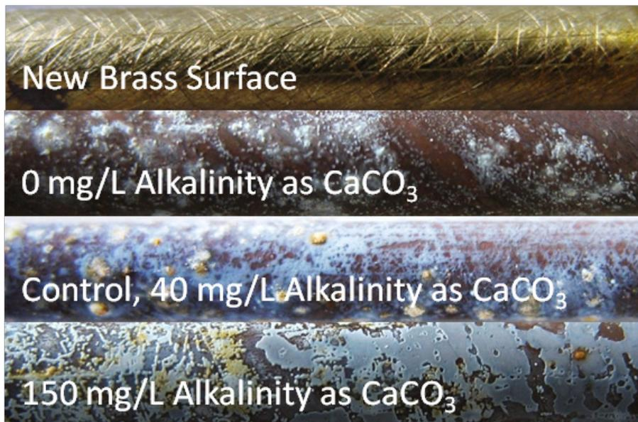
Figure 4 – 7 Surface images for the new brass surface, the low alkalinity, the control and the high alkalinity conditions
