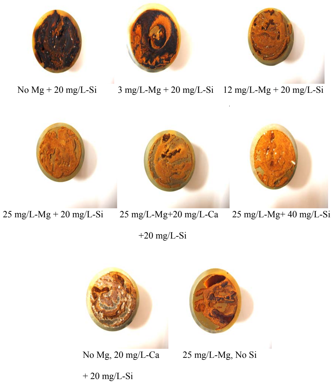
Figure A-1-15: Scale morphology after 37 days exposure, no SRB added.
