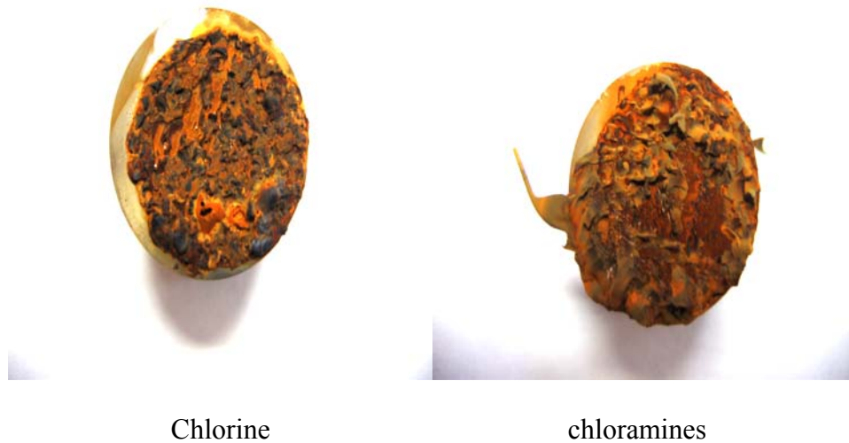
Figure 1-15: Scale morphology after 46 days exposure, no SRB inoculation.
