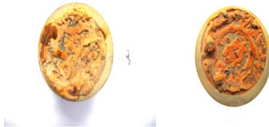
Figure A-1-13: Scale morphology after 153 days exposure (old coupons) and 118 days exposure (new coupons), SRB inoculated.
