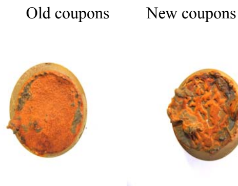
Figure 1-14: Scale morphology, highest sulfate, chloramines, SRB inoculated.
